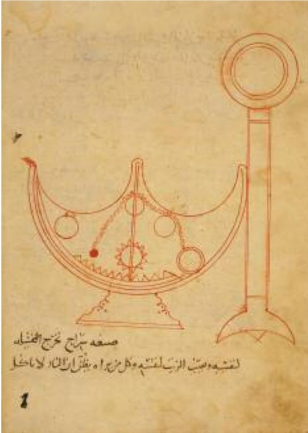
Fig. 2: Self-feeding lamp of the Banū Mūsā, Model No. 96 in the Manuscript MS 559/9, Staatsbibliothek zu Berlin C Preußischer Kulturbesitz, Oriental Department. At the centre is the gear wheel, which maintains the supply of oil to the wick; at the top left above the circle is the opening where the oil is poured in.
