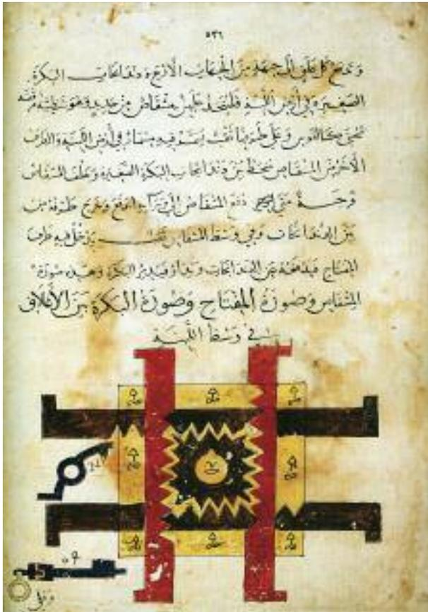
Fig. 5: A lock for locking a chest by means of a combination of letters and numbers. From al-Jazari, *Compendium on the Theory and Practice of the Mechanical Arts*. Reproduction by the Institute for the History of Arabic-Islamic Science Frankfurt am Main, 2002.
